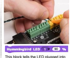
This block tells the LED plugged into LED connector #1 to turn on at 90% brightness.
